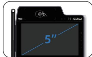
Sensitive screen to capture finger and stylus-based signature.
